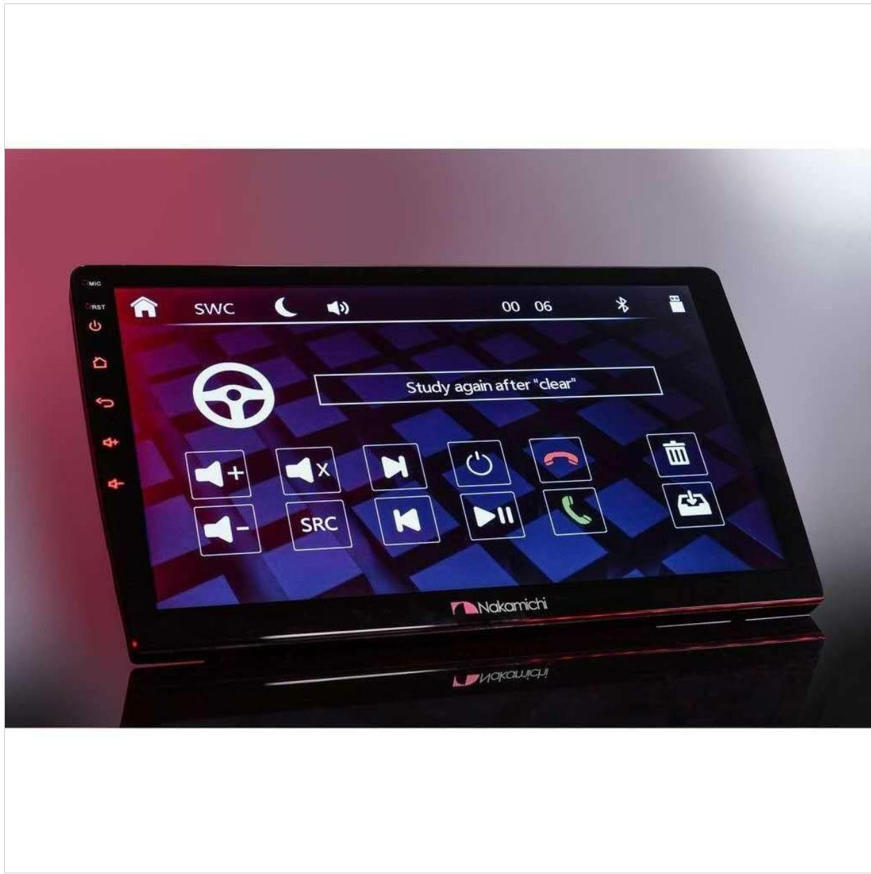
**Figure 6.1:** The steering wheel control learning interface, allowing users to program physical steering wheel buttons to control the stereo functions.
