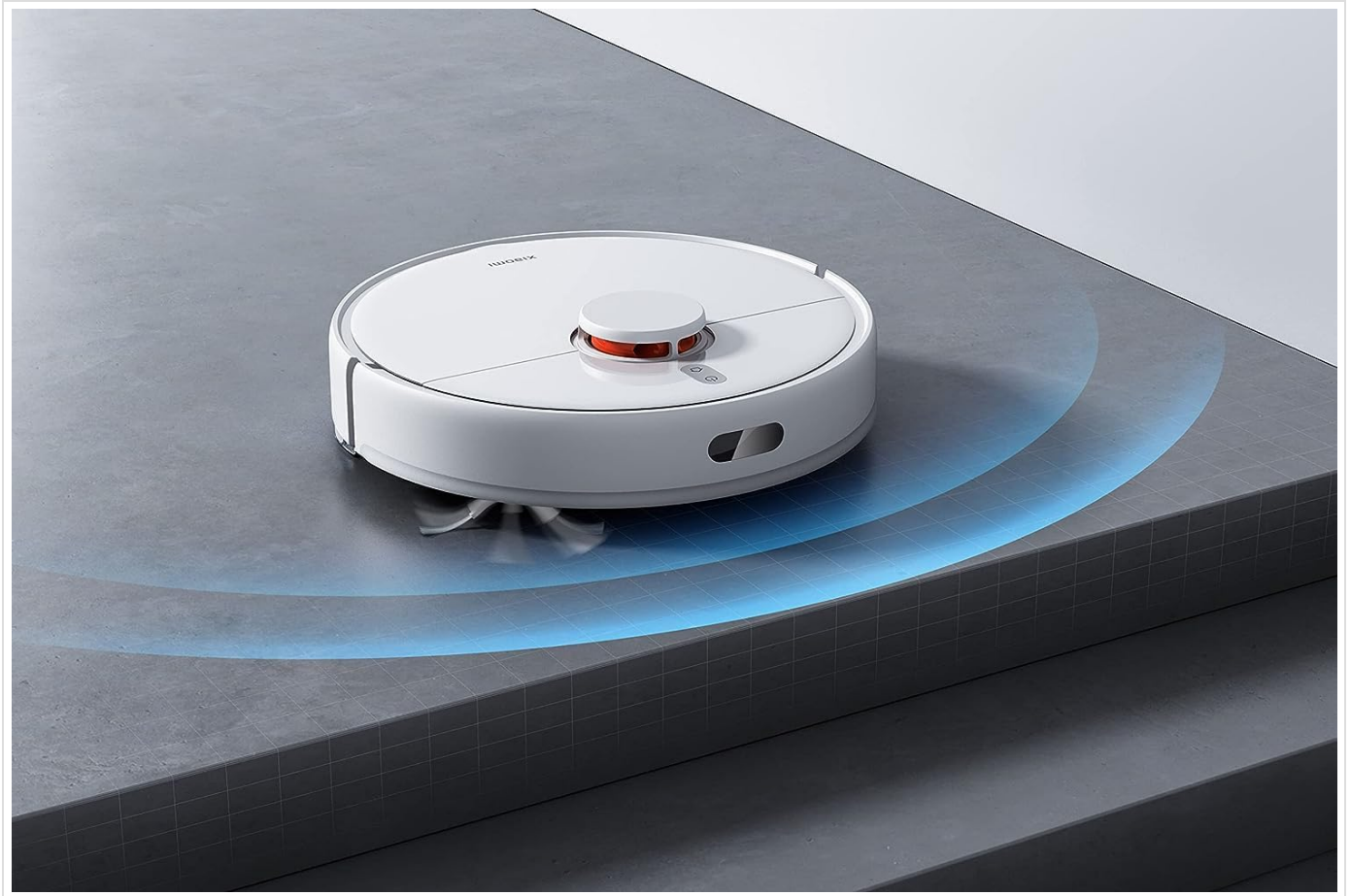
Figure 8: The Xiaomi Robot Vacuum X10 demonstrating its navigation capabilities, approaching a raised surface or step, indicating its ability to detect and avoid obstacles or drop-offs.
