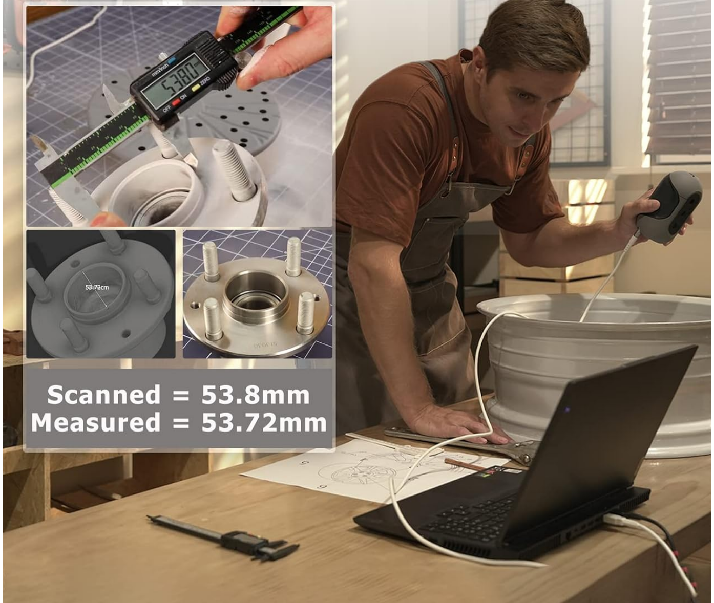
Figure 2.1: Illustration of the Mole scanner's 0.1mm accuracy in recreating object dimensions.
