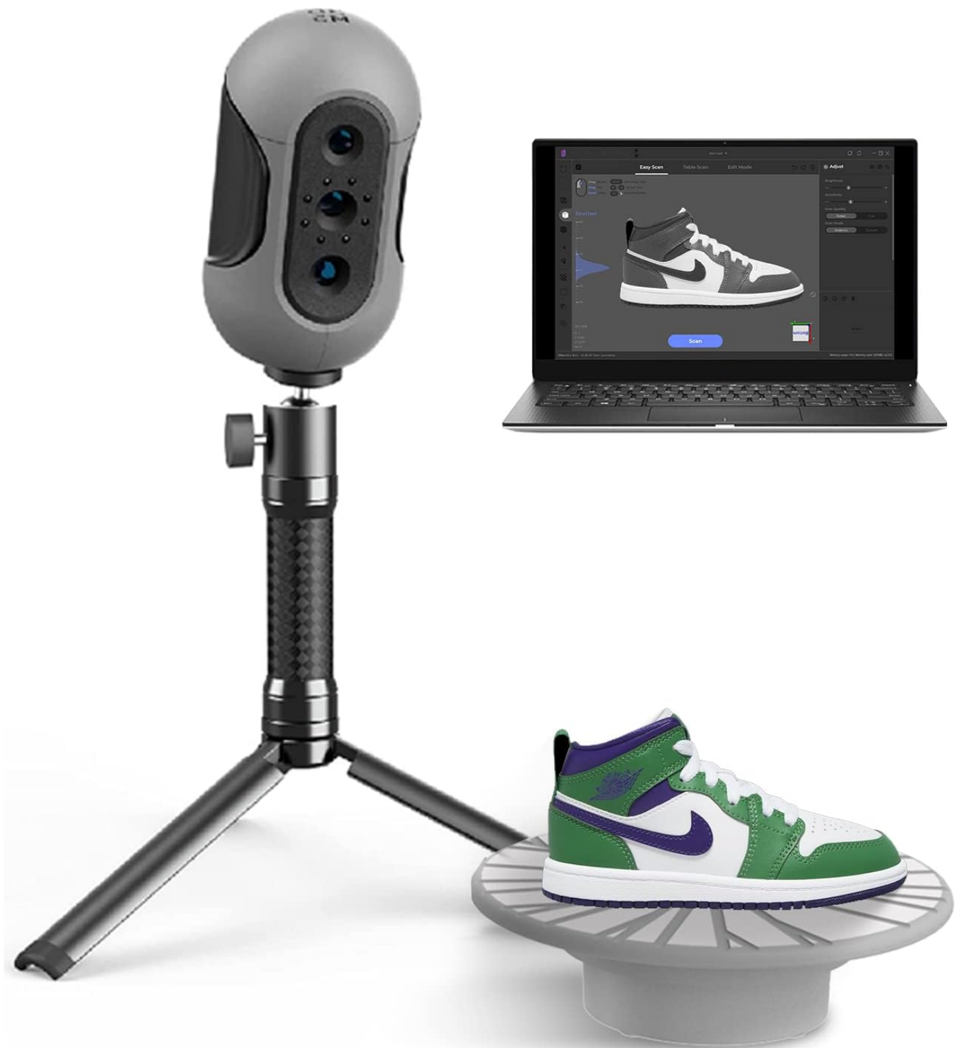
Figure 1.1: The Mole 3D Scanner setup, including the scanner unit, tripod, turntable, and a laptop running the scanning software.
