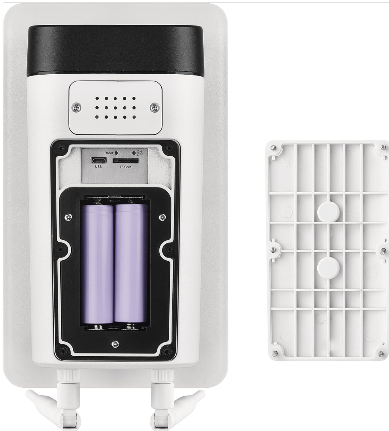
Image 3.1: View of the camera's battery compartment, USB port, and TF (microSD) card slot.
