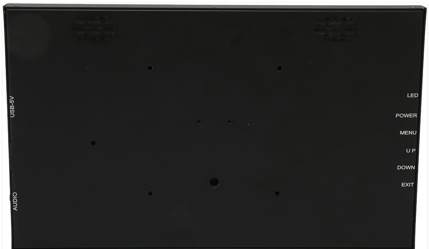
Figure 4: Side view of the monitor, illustrating the location of the ports and control buttons.
