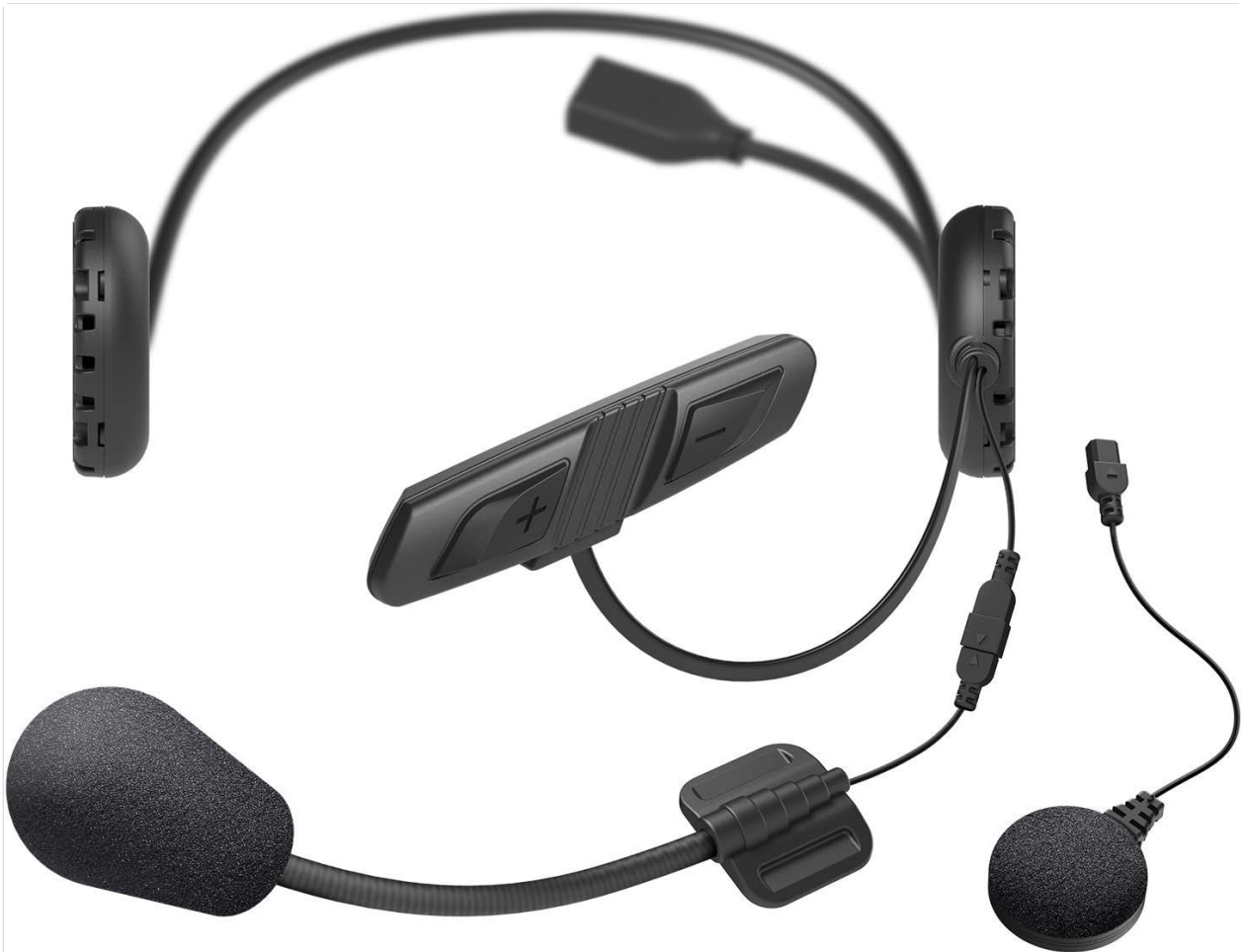
Image: All components of the Sena 3S Plus Universal headset, including the main unit, microphones, speakers, and various fasteners and cables.
