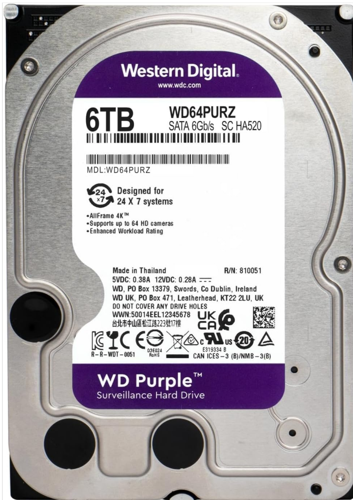
Figure 2: Back view of the WD Purple 6TB Surveillance Hard Drive. This image displays the drive's metallic casing and the product label, which includes the model number WD64PURZ, SATA 6 Gb/s interface details, and certifications.
