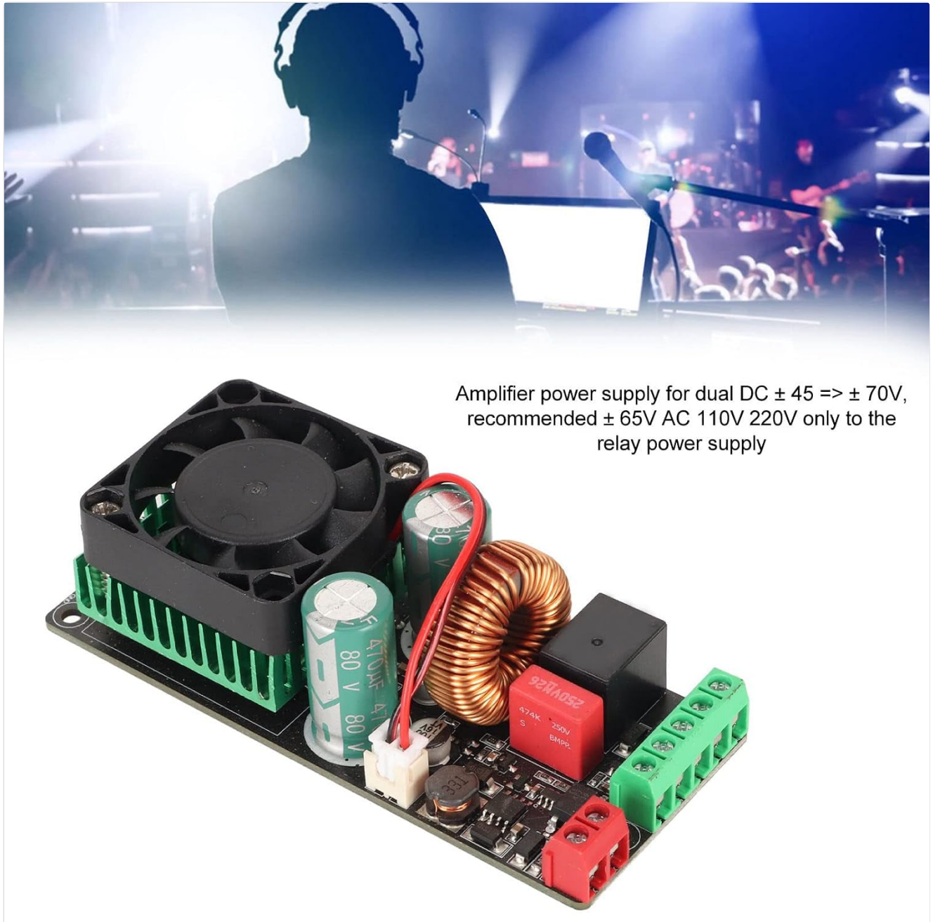
Figure 4: Power supply requirements. This image indicates that the amplifier power supply is for dual DC \pm 45\text{V} to \pm 70\text{V} , with a recommended \pm 65\text{V} . It also notes that AC 110V/220V is only for the relay power supply.
