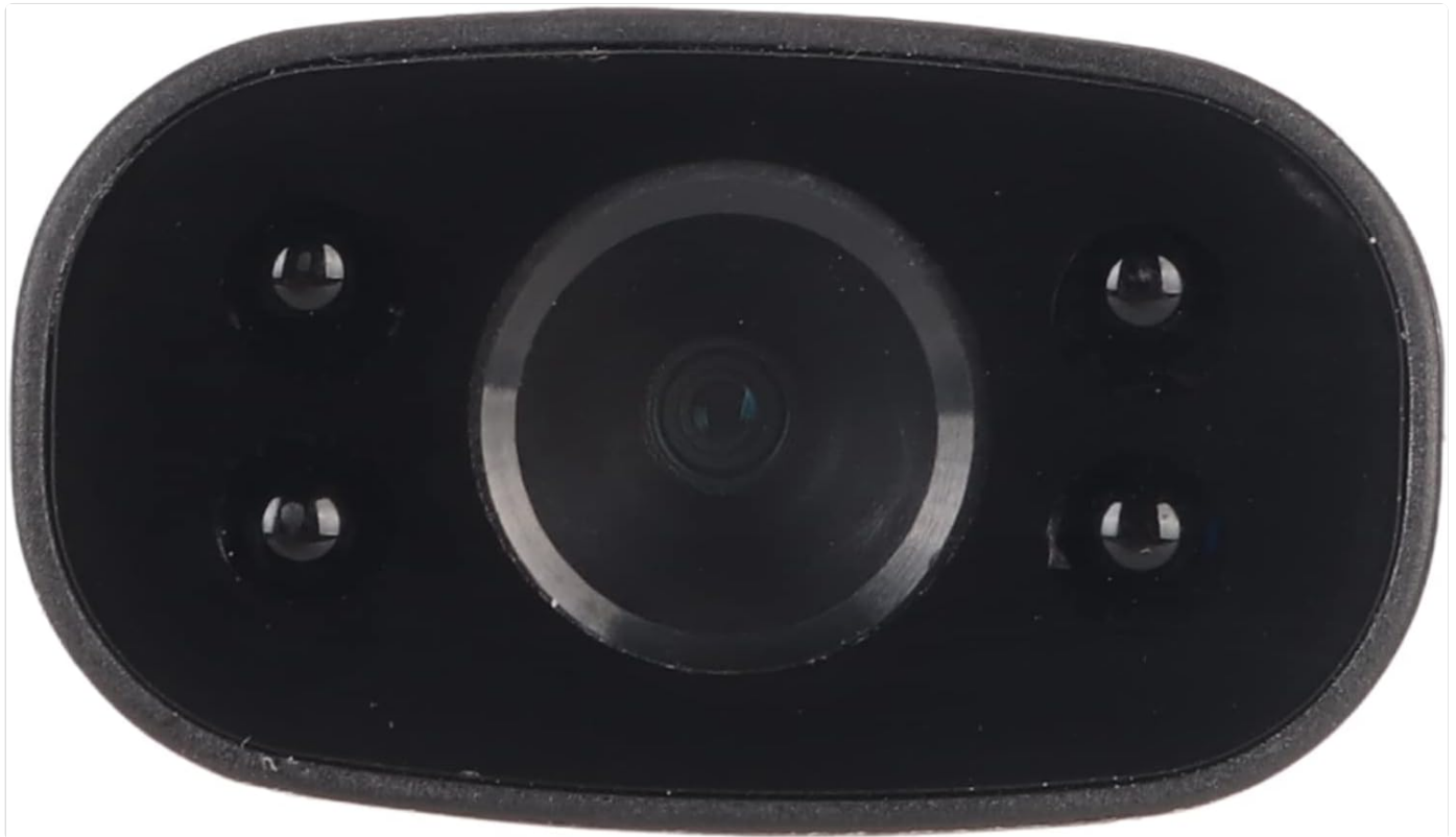
Image 5.2: Front view of the camera, detailing the lens and infrared LED lights for night vision.
