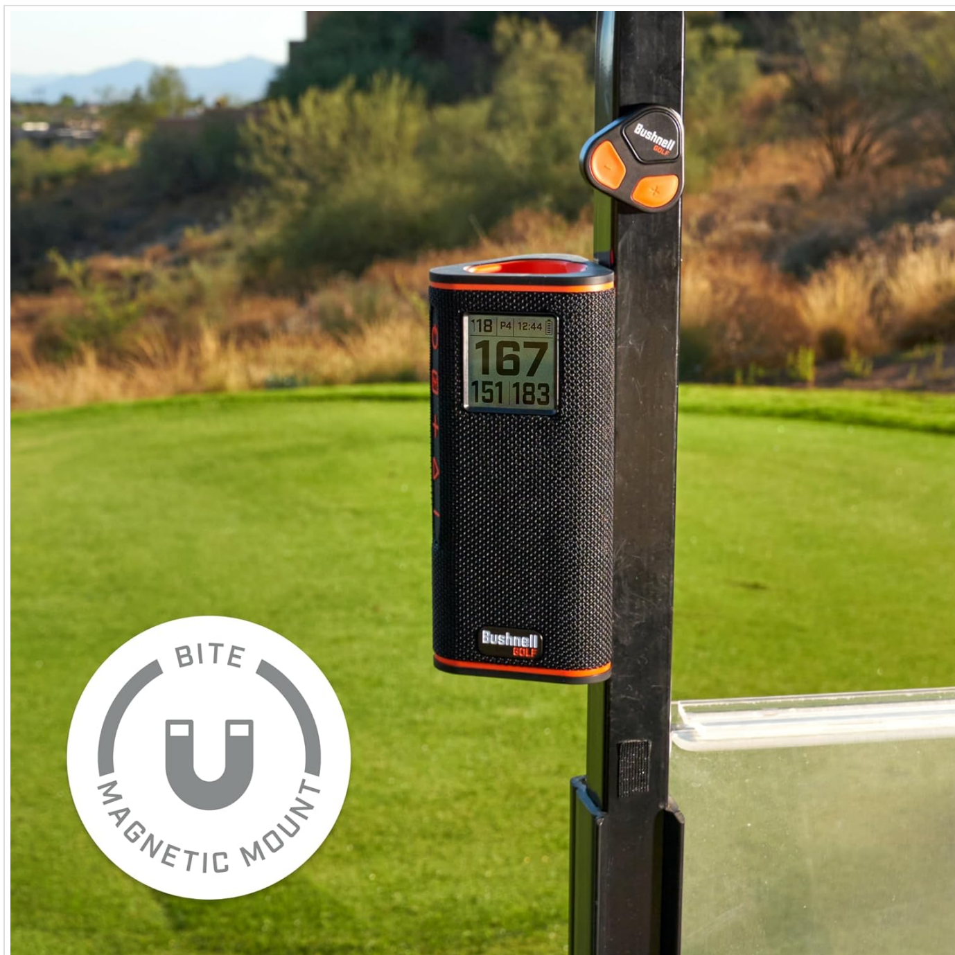
Image: The LCD screen of the Wingman View showing distances to the front, center, and back of the green, along with hole and par information.
