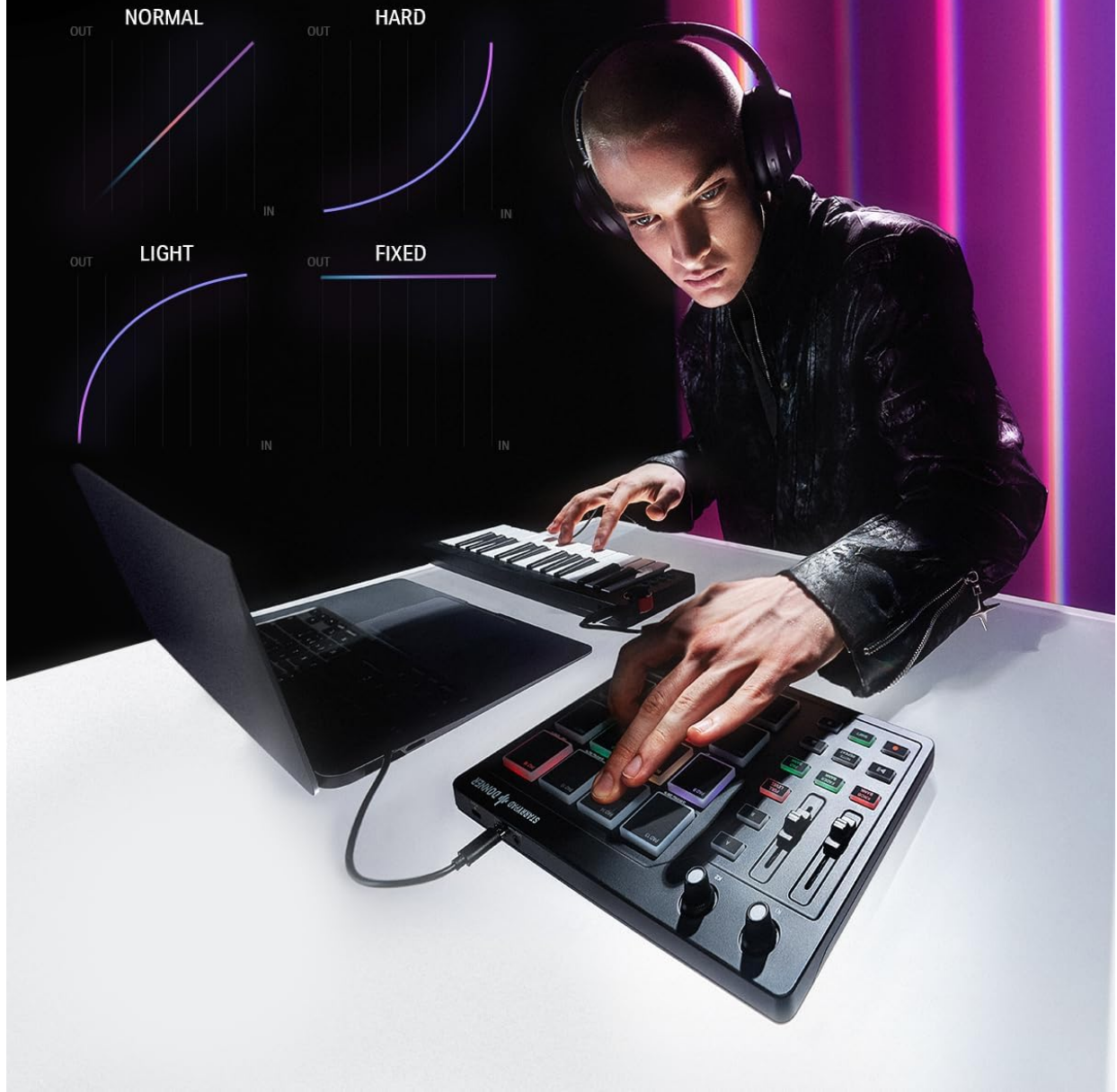
Image: Visual representation of the four velocity sensitive curves (Normal, Hard, Light, Fixed) available on the STARRYPAD DPD-16, catering to diverse performance needs.
