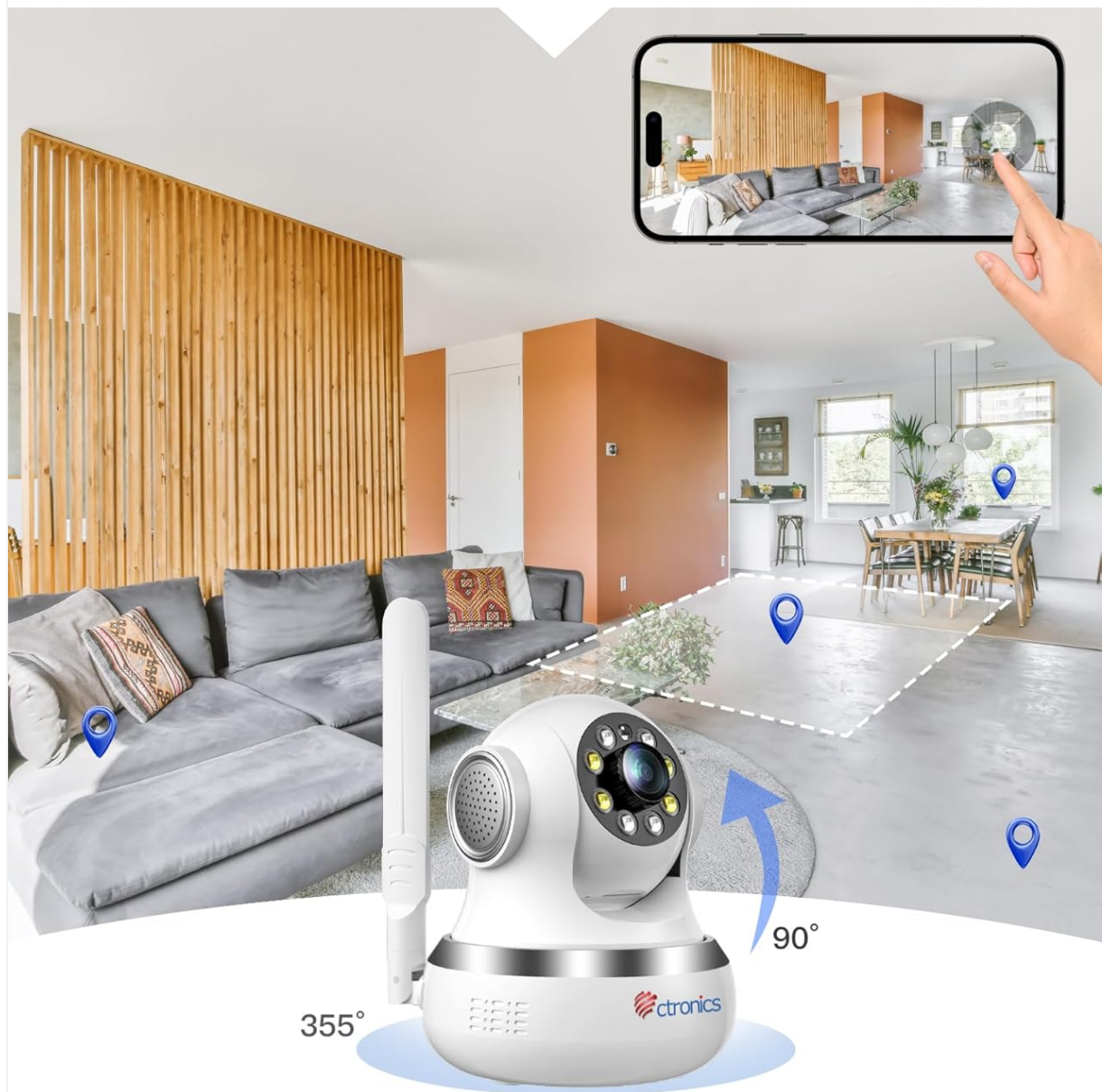
Figure 4.2: Visual representation of the camera's 355-degree horizontal rotation and 90-degree vertical tilt capabilities.
