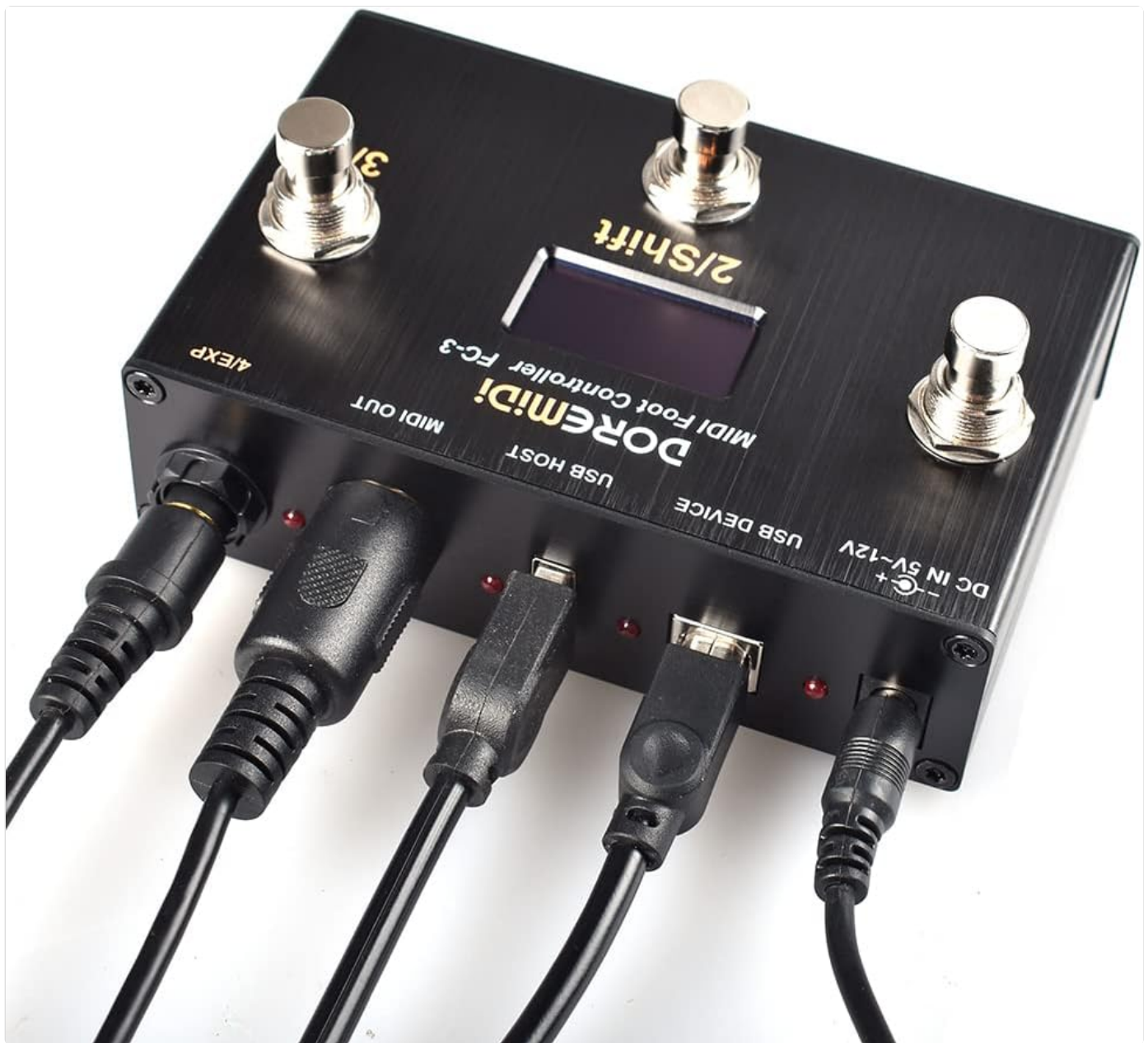
Figure 2: Side view of the FC-3 with cables connected, providing a clearer view of the port labels and cable types.
