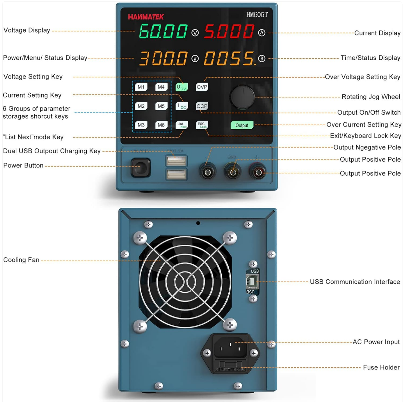
Figure 2.1: Front and Rear Panel Layout. This image illustrates the various controls and ports on the front and back of the HM605T power supply, including the display, control buttons, output terminals, USB ports, cooling fan, and AC power input.
