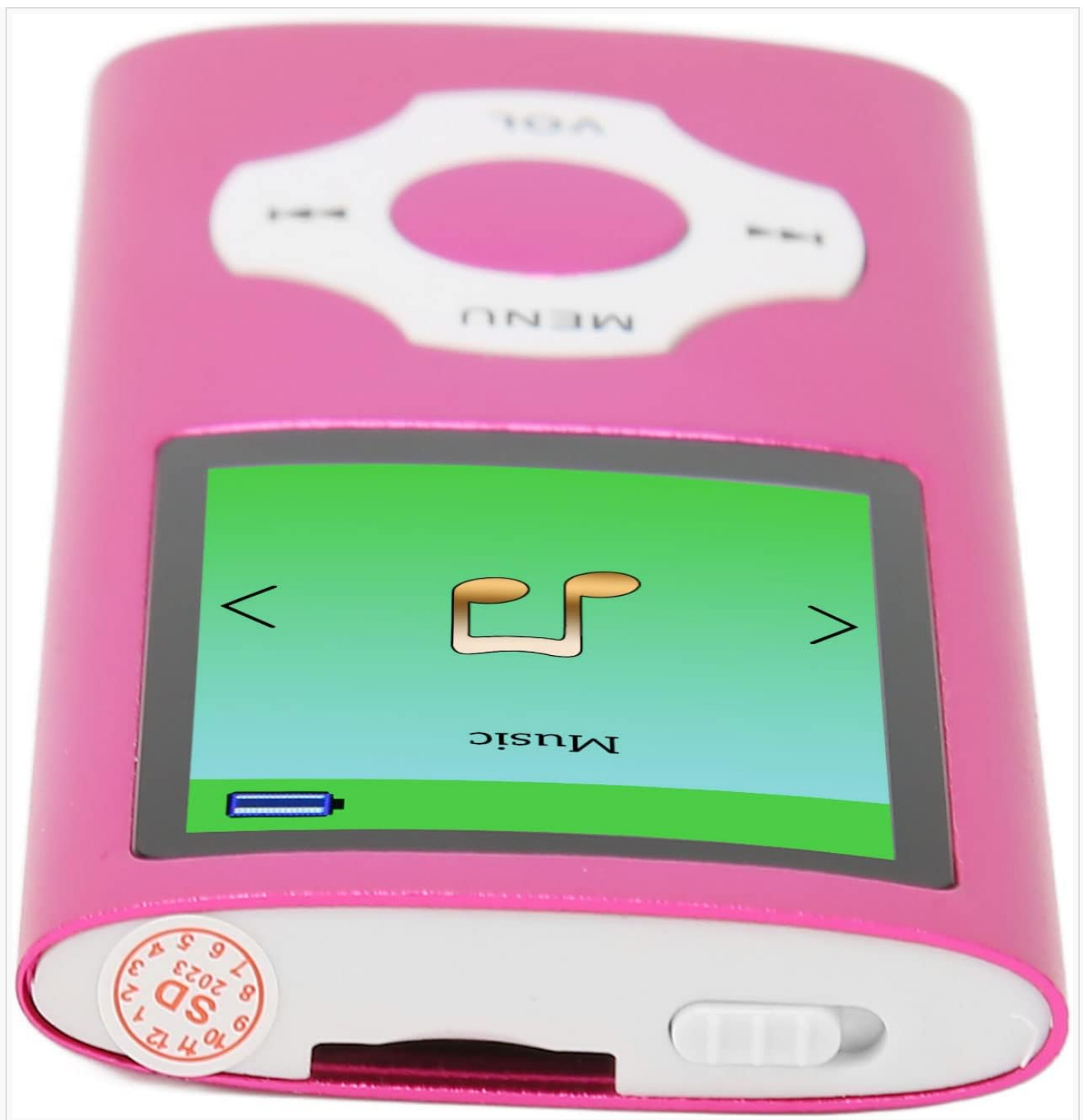
Image: Side view of the Dpofirs MP3 player, showing the slot for a Micro SD memory card.
