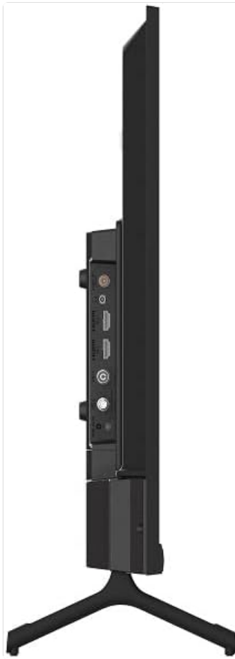
Figure 3.2: Close-up of the side panel showing the various input and output ports available on the television.
