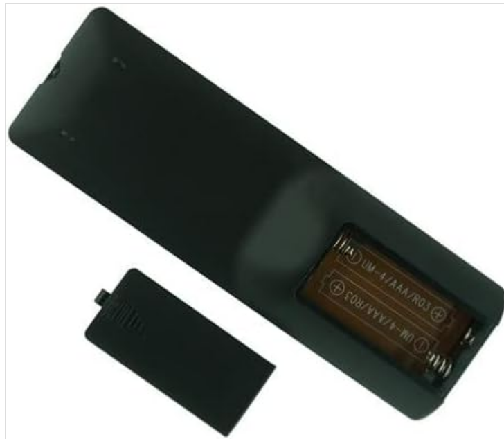
Image: The remote control with its battery compartment open, showing where to insert the two AAA batteries according to polarity markings.
