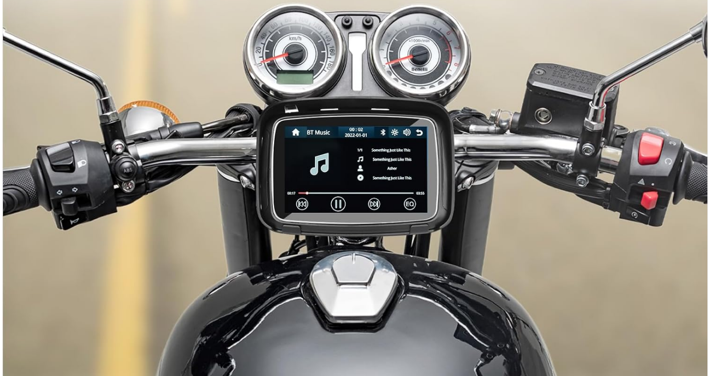
Figure 5.3: Bluetooth interface on the navigator, demonstrating phone call and music playback options.
