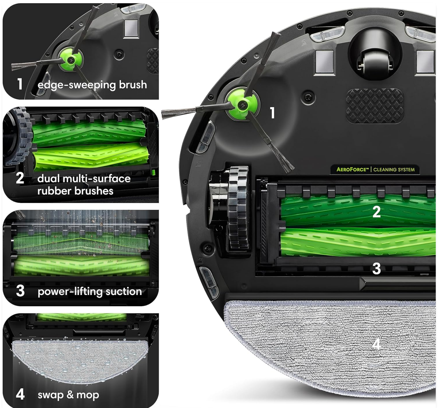
Image: An underside view of the Roomba Combo i5+ robot, highlighting its edge-sweeping brush, dual multi-surface rubber brushes, power-lifting suction area, and the mop pad, illustrating the components of its 4-stage cleaning system.
