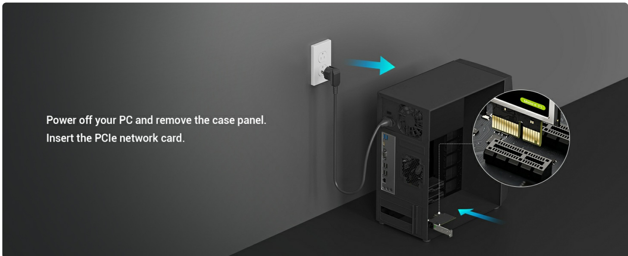
Image: Illustration of powering off the PC, removing the case panel, and inserting the PCIe network card.
