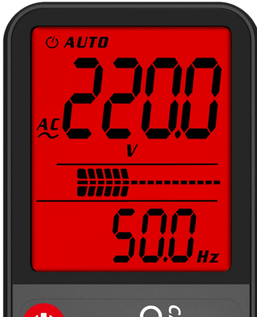
Image: A close-up of the BSIDE S7 Multimeter's display, illustrating its 3-line output which simultaneously shows voltage, frequency, and an analog bar for comprehensive test results.
