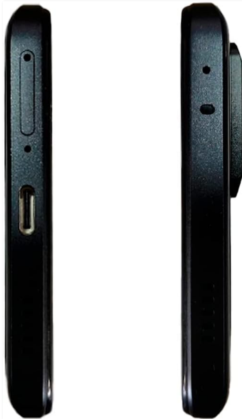
Image 3.2: Left side view of the Poco F5 Pro, showing the SIM card tray and USB-C charging port.
