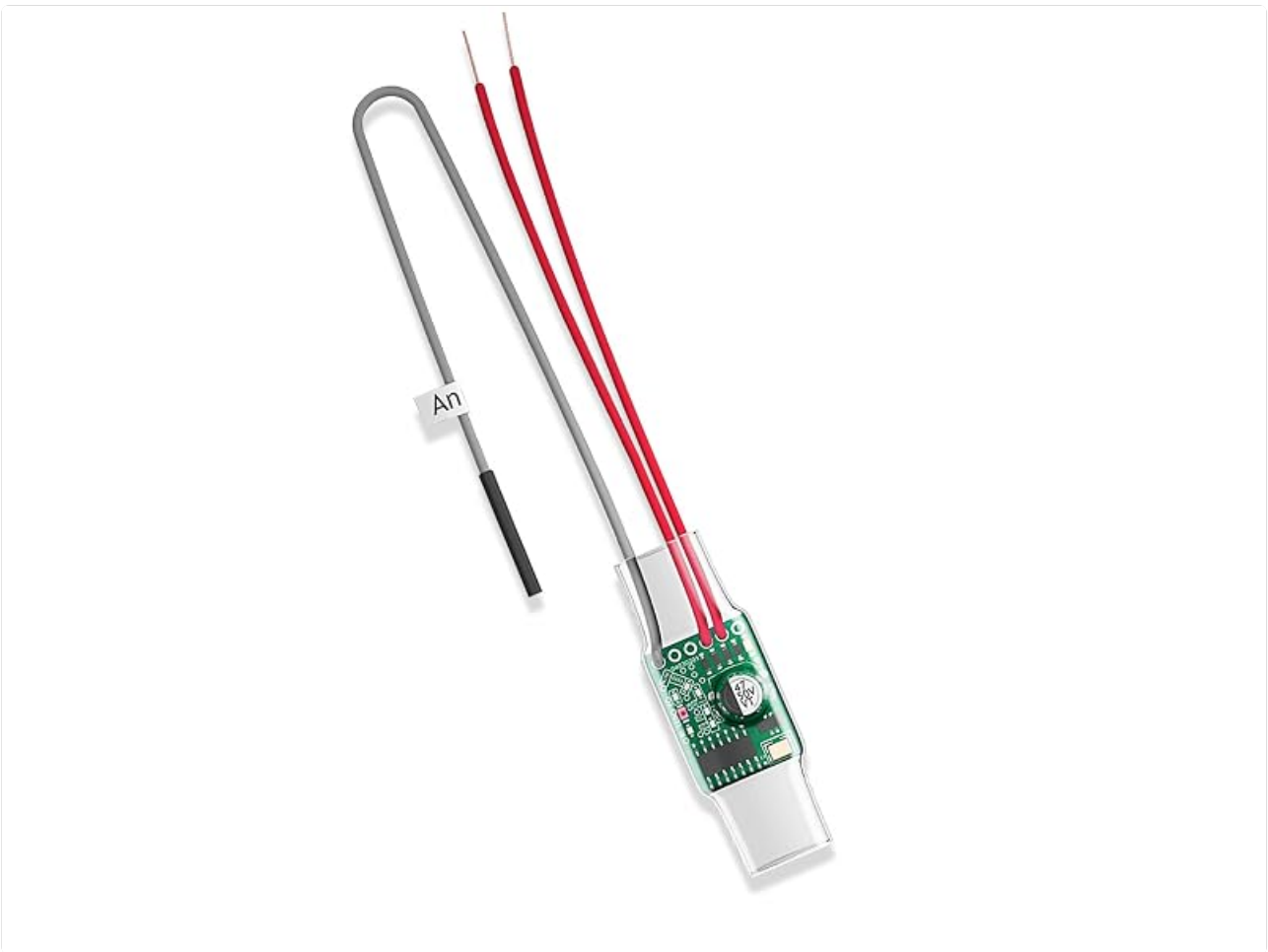
Image: A close-up view of the compact wireless converter module with its antenna and power/signal wires. This small unit is designed to fit discreetly within your existing doorbell housing.
