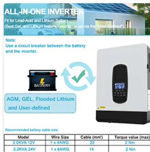
Image 4.2: Battery compatibility and recommended cable sizes. For 2.2KVA-12V, use 1 x 4AWG cable (22 mm 2 ) with a maximum torque value of 2 Nm.
