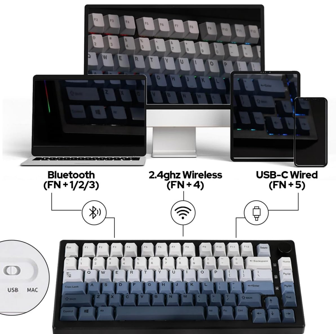
Image: Overview of the three connectivity modes: Bluetooth (FN+1/2/3), 2.4GHz Wireless (FN+4), and USB-C Wired (FN+5).
