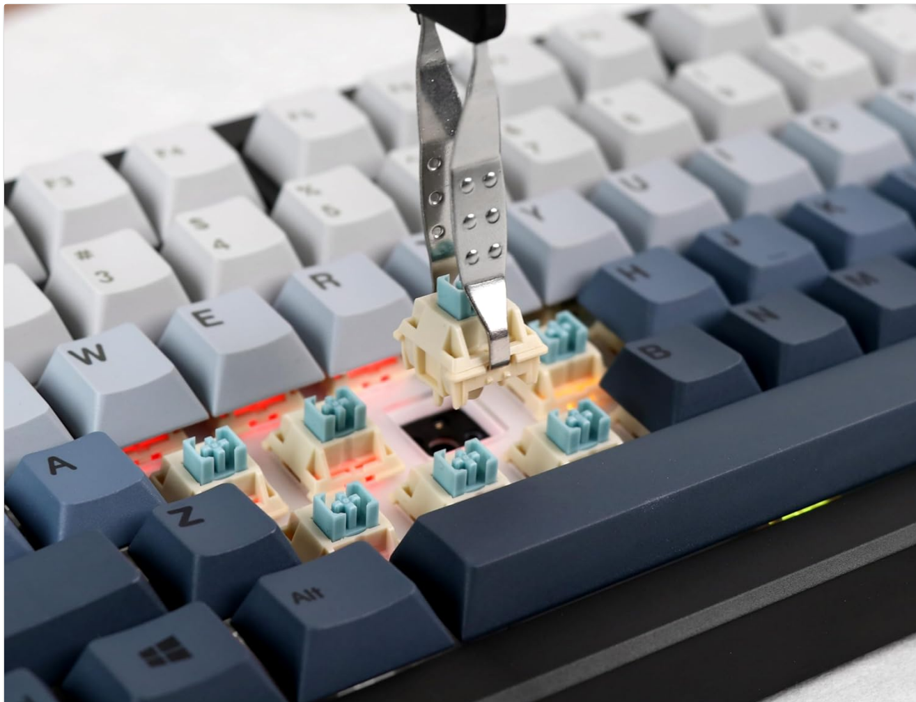
Image: Proper installation of a mechanical switch into the hot-swappable PCB.
