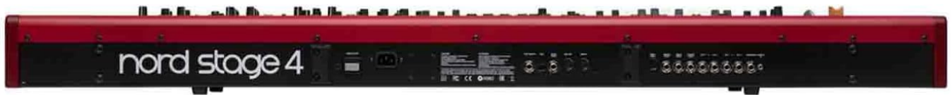
Figure 8.2: Rear view of the Nord Stage 4, highlighting the various input and output connections including power, audio, USB, and MIDI ports.
