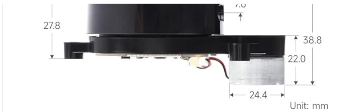
Image: Technical drawing showing the outline dimensions of the D200 LiDAR unit in millimeters.
