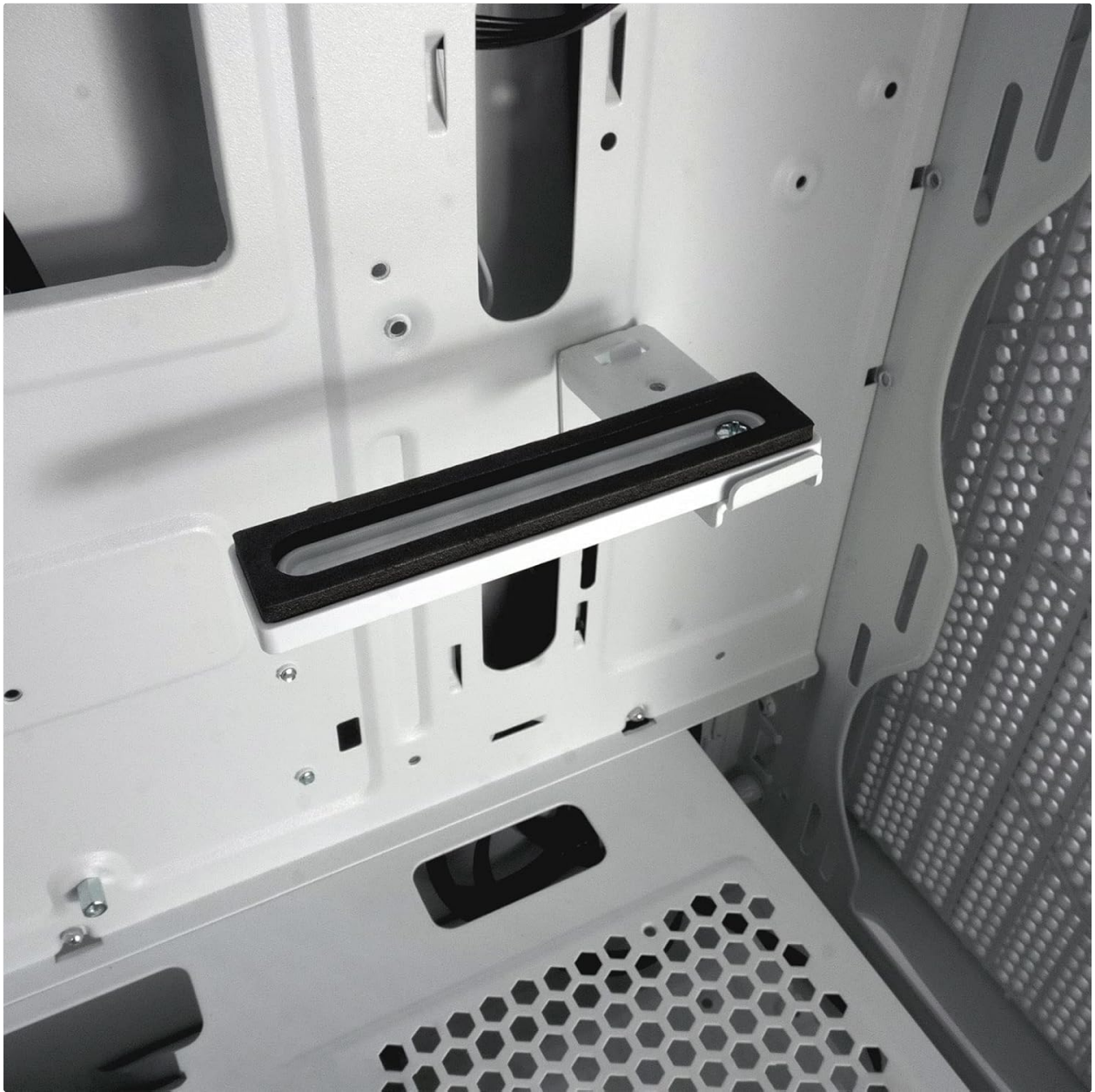
Figure 4: GPU support bracket for graphics card stability.
