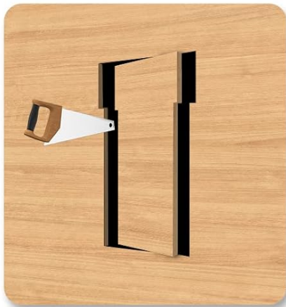
Step4: Saw the marked door along the hole
