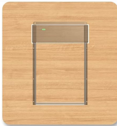
Step2: Mark the hole locations for the door
