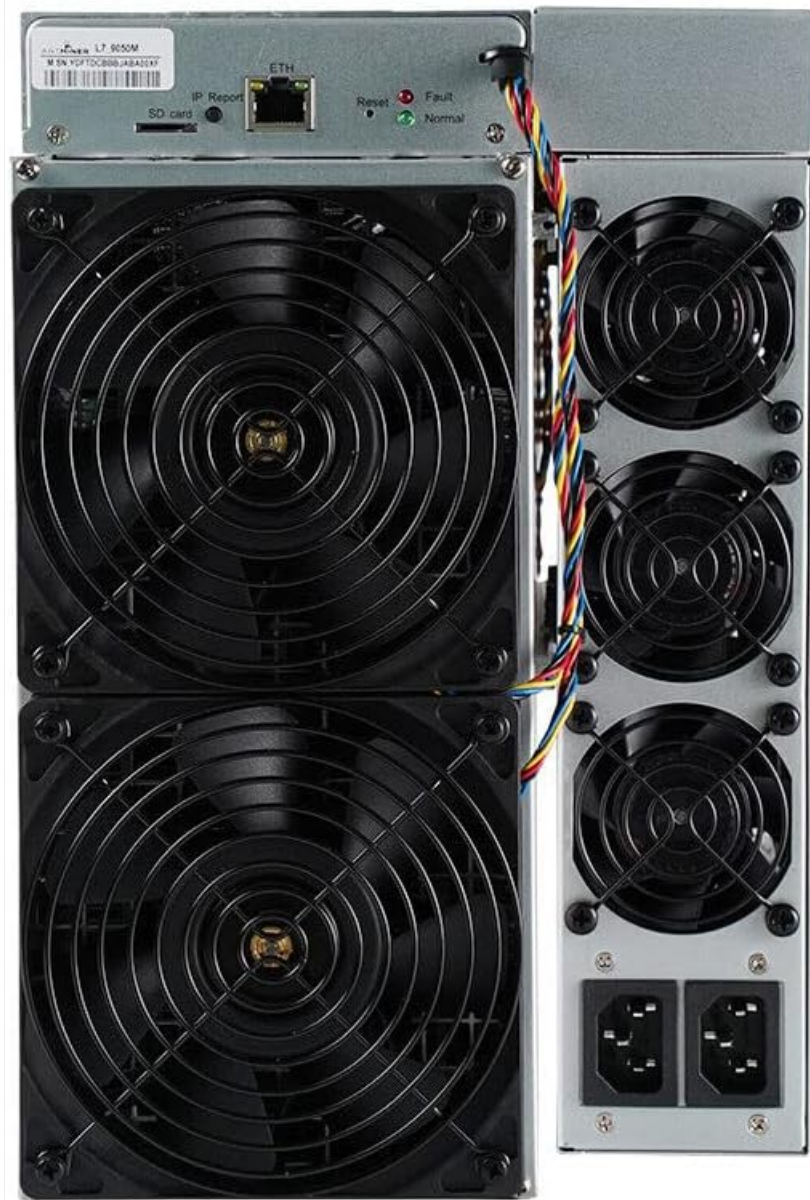
Figure 4.3: The rear panel of the Antminer L7, featuring the dual power input ports and the exhaust fans for cooling.
