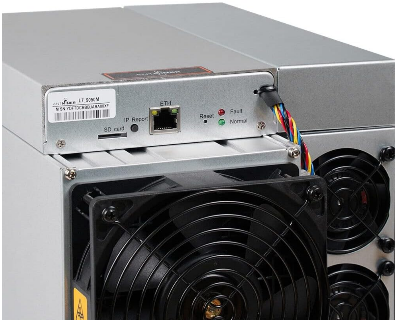
Figure 4.4: A detailed view of the control board, including the Ethernet port, IP Report button, Reset button, and the Fault and Normal indicator LEDs, along with an SD card slot.
