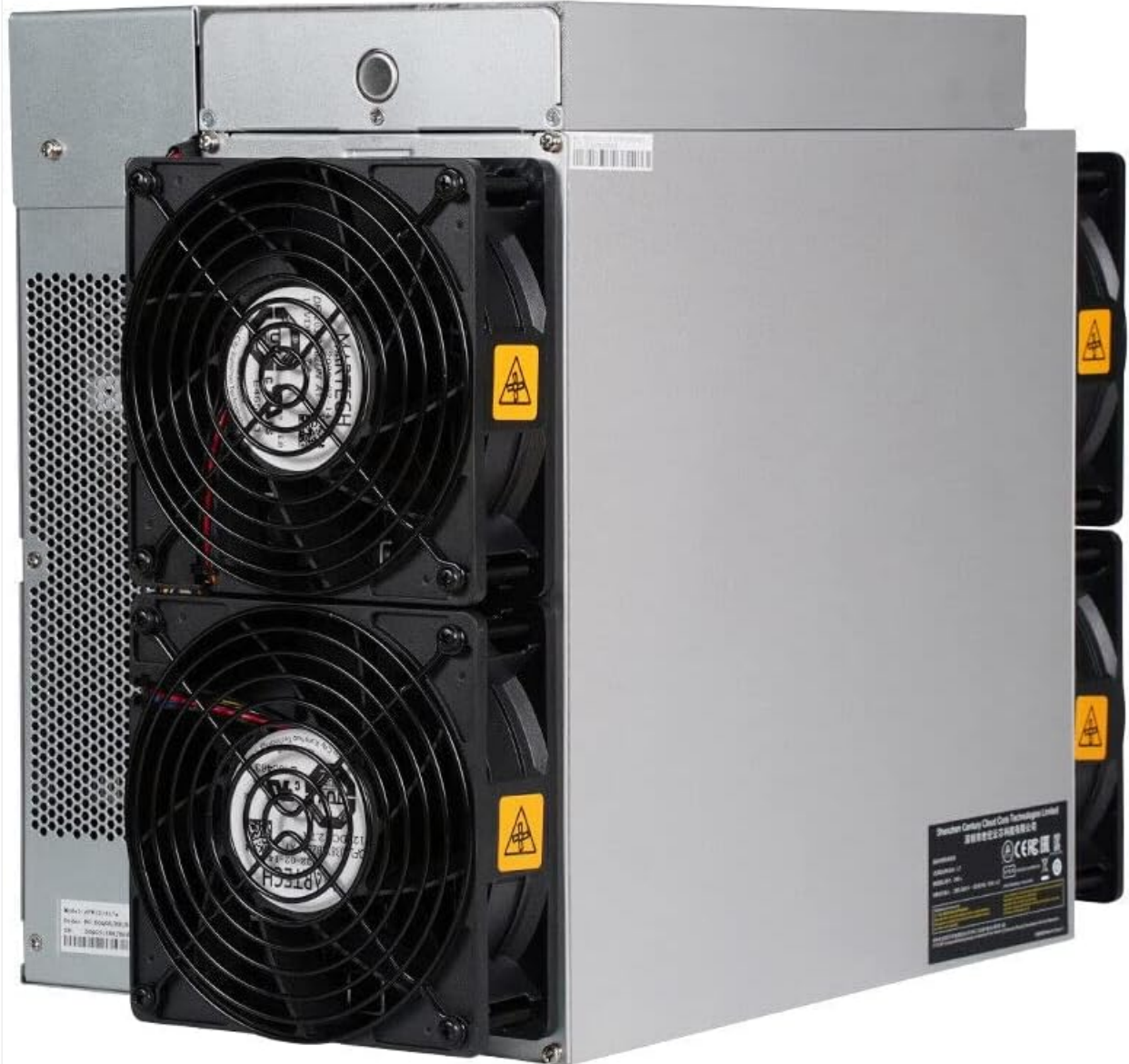
Figure 4.2: A side perspective of the Antminer L7, illustrating the arrangement of its cooling fans and the overall chassis design.
