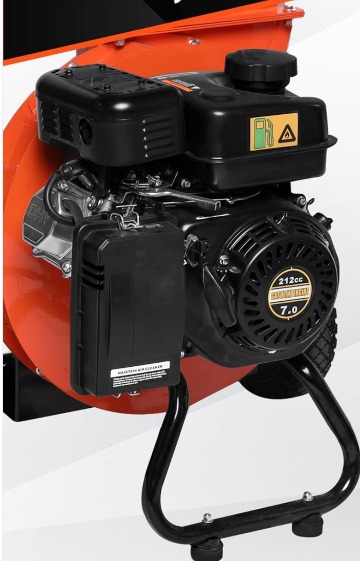
Figure 4: Close-up of the 7HP 212cc engine, showing the recoil starter and low oil alert sensor.
