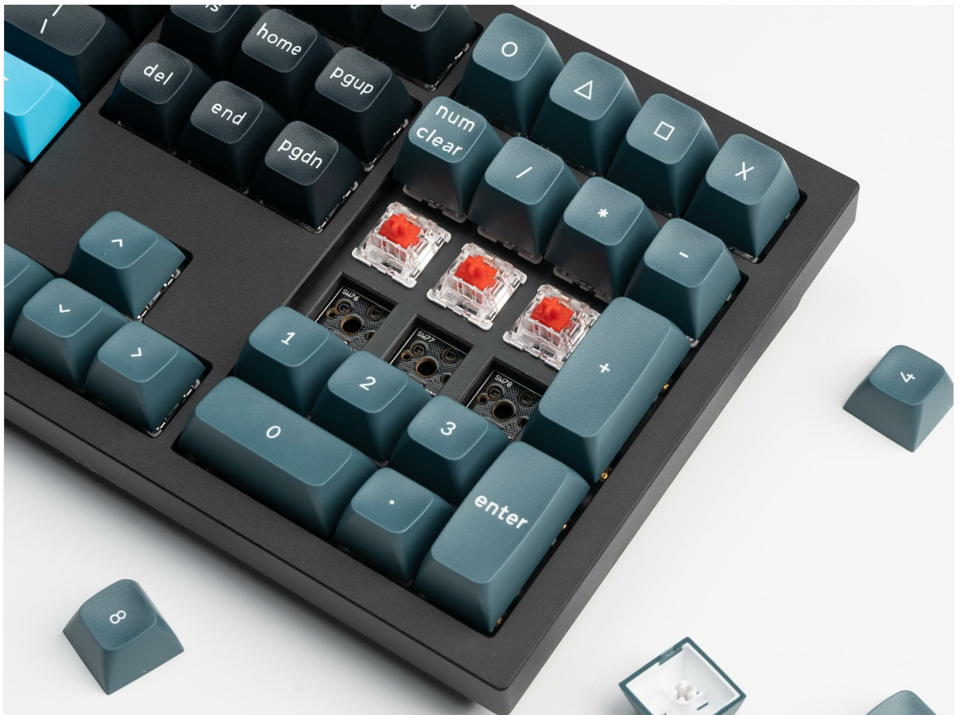
Image 5.1: Demonstrating the hot-swappable feature of the Keychron Q6 Pro, showing switches being removed and inserted.
