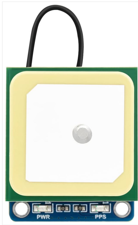
Image: Top view of the LC76G GNSS module, showing the ceramic antenna.
