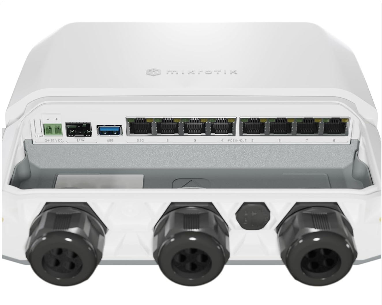
Figure 4.3: A close-up view of the MikroTik RB5009UPr+S+OUT router with its protective cover open, revealing the Ethernet ports, SFP+ port, USB port, and DC input terminal.
