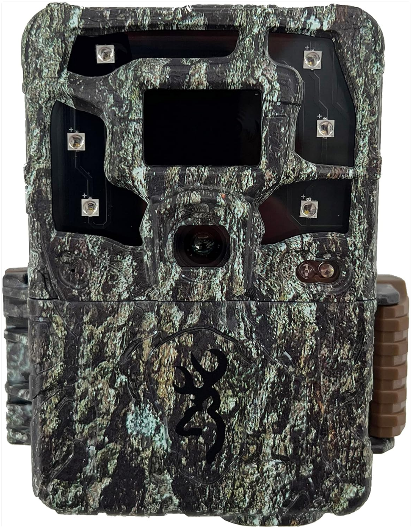
Image: Front view of the trail camera, highlighting the lens, IR emitters, and motion sensor.
