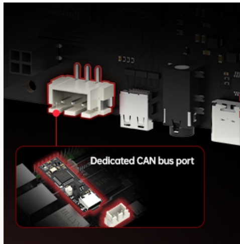
Image 5.3: The BTT Pi V1.2 board with support for CAN Bus connectivity.
