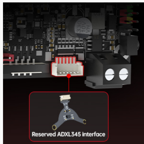
Image 5.2: Close-up of the reserved ADXL345 interface on the BTT Pi V1.2 motherboard.
