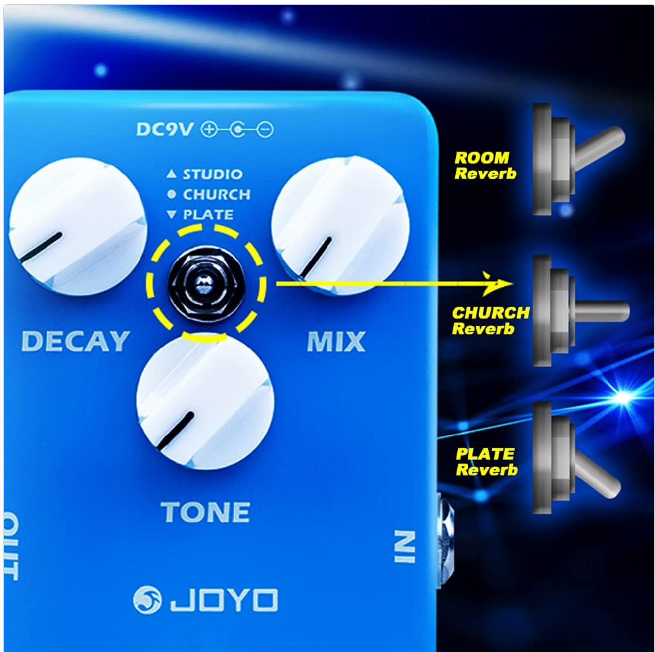
Image: A close-up view of the JOYO JF-20 MOIST REVERB pedal's controls. The image highlights the Decay, Mix, and Tone knobs, as well as the three-position toggle switch for selecting Studio, Church, or Plate reverb modes.
