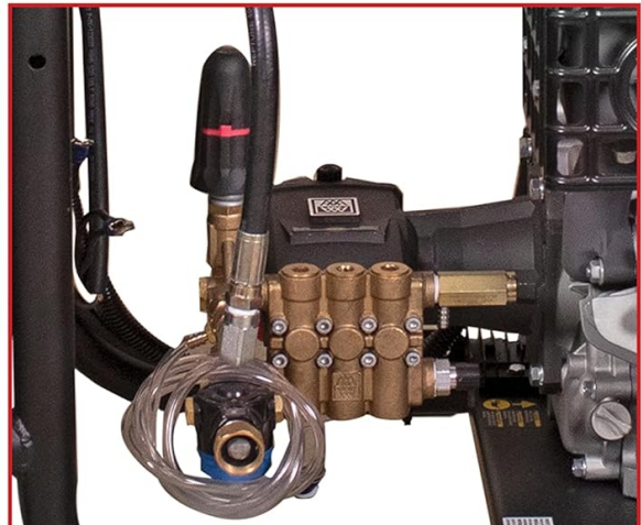
AAA® industrial triplex pump built with external unloader and bypass hose
