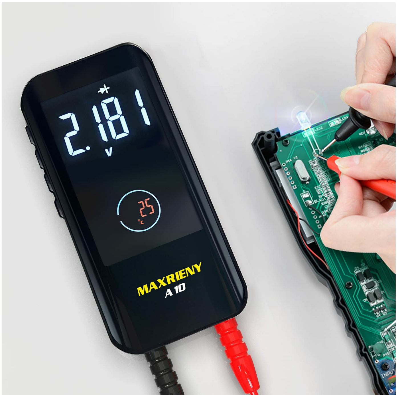
Figure 6.3: Performing a Diode Test
