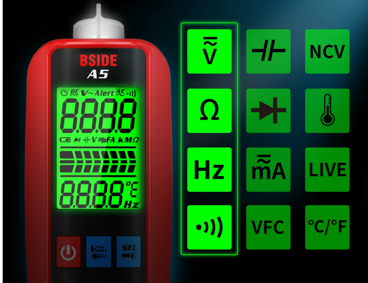
Image: The BSIDE A5 display showing icons for various measurement modes, highlighting its auto-selection capability.
