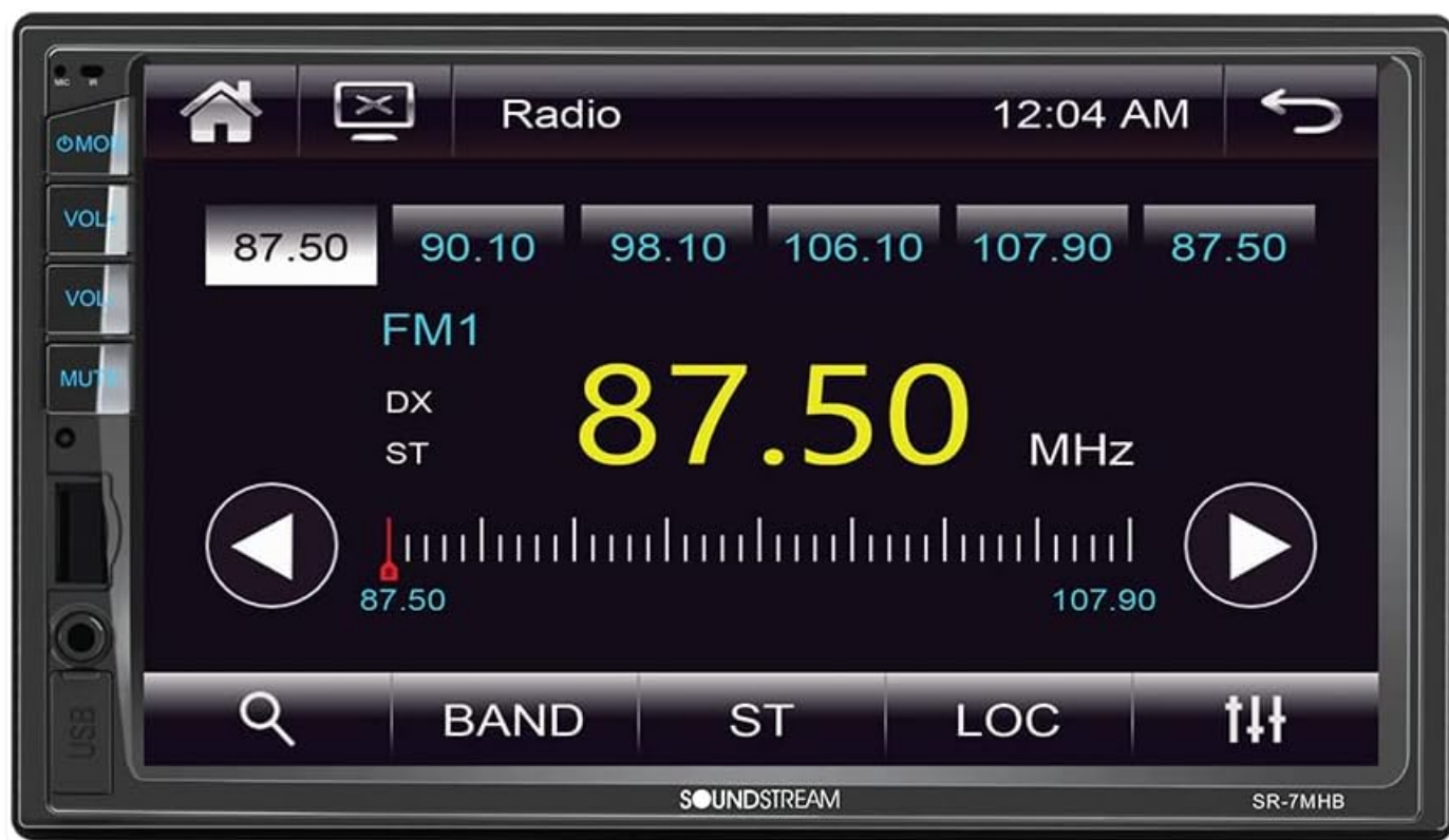
Image: The front of the Soundstream SR-7MHB unit, highlighting the large 7-inch touchscreen display currently showing the radio tuning interface. On the left side, physical buttons for mode, volume up/down, and mute are visible, along with a USB port at the bottom left.
