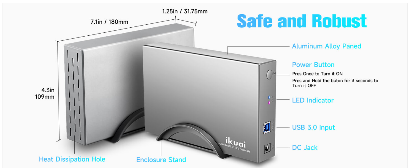
Image: A detailed view of the enclosure highlighting its aluminum alloy panel, power button, LED indicators, USB 3.0 input, DC jack, heat dissipation holes, and enclosure stand. Dimensions are also provided.
