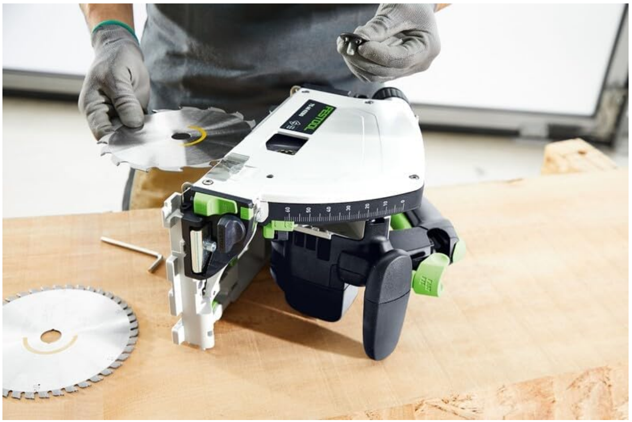
Figure 4.1: Demonstrating the process of changing the saw blade using the integrated hex key and FastFix spindle lock.
