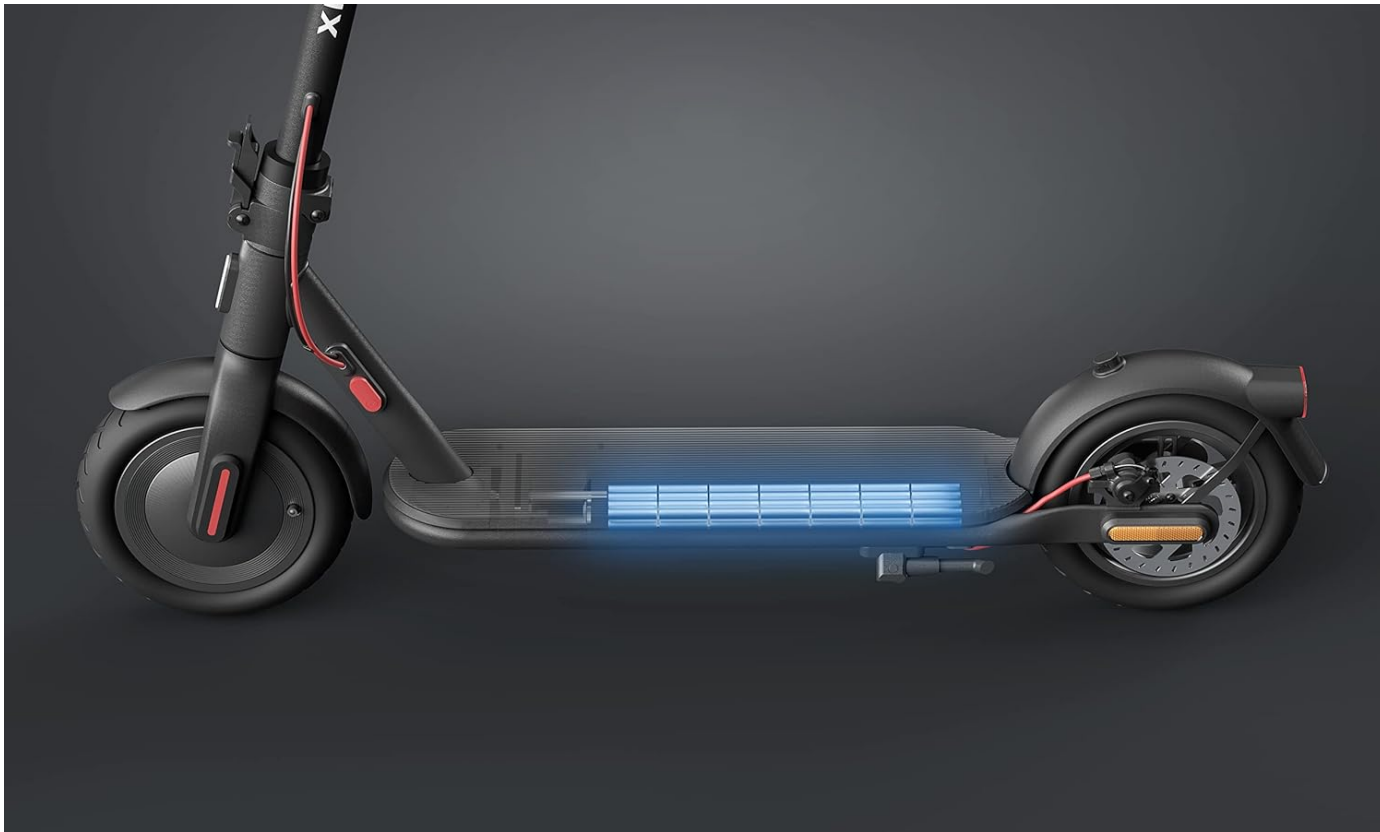
Image: An internal view illustrating the battery pack within the scooter's deck.
