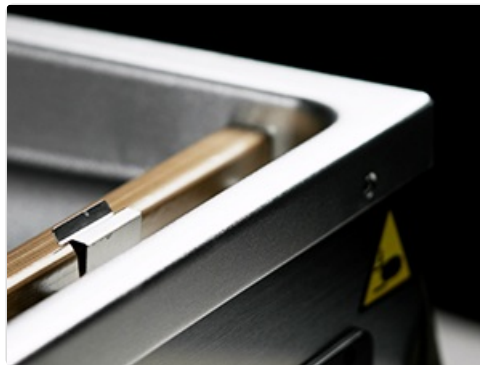
Figure 4.1: Close-up view of the vacuum chamber interior, highlighting the seal bar in position.
