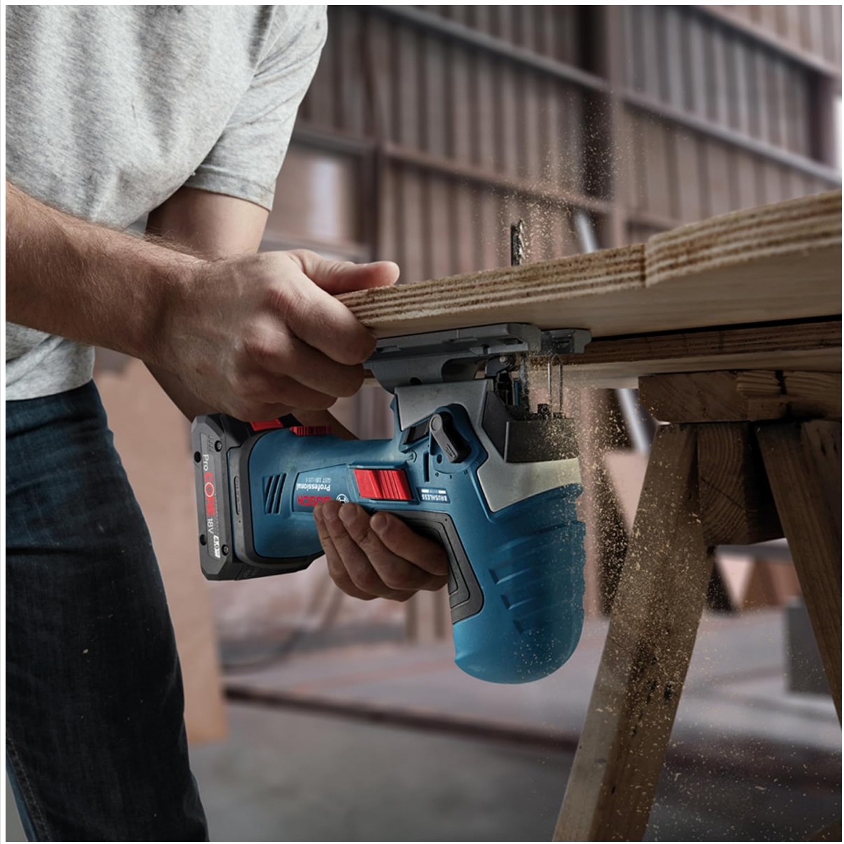
Figure 4: Close-up view of the Bosch Professional Jigsaw blade cutting wood. This image provides a detailed look at the cutting action and the dust blower keeping the line clear.
