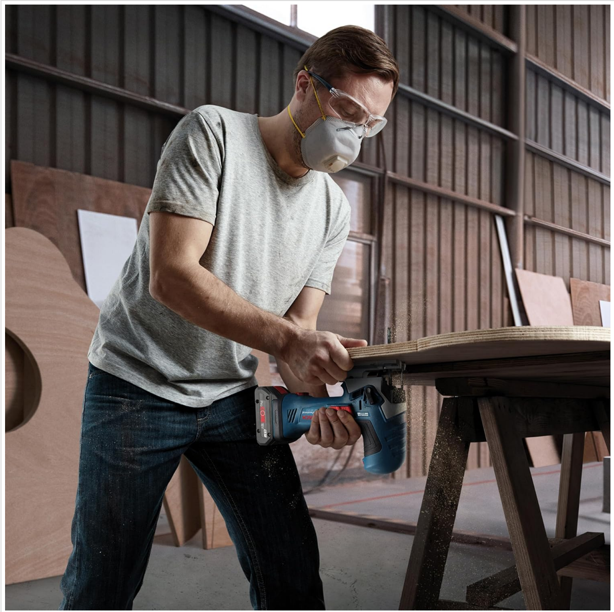
Figure 3: User operating the Bosch Professional Jigsaw for a cross cut. This image illustrates the tool's capability for straight cross cuts across a wooden panel.
