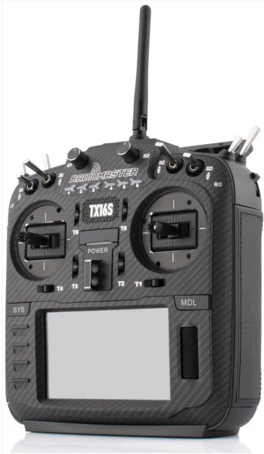
Figure 3.2: Angled front view of the TX16S Mark II MAX Edition. This perspective showcases the ergonomic design, including the textured side grips and the placement of the various switches and gimbals, providing a better understanding of the user interface layout.
