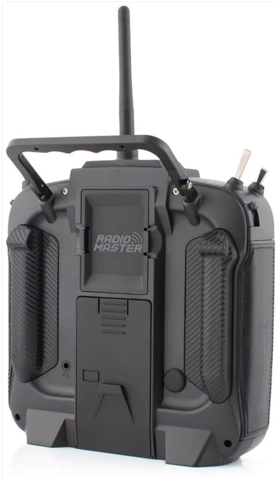
Figure 3.4: Rear view of the TX16S Mark II MAX Edition. This view highlights the redesigned battery cover for improved access, the JR compatible module bay, the rear-mounted audio jack, and the rear DIY socket for personalized modifications.
