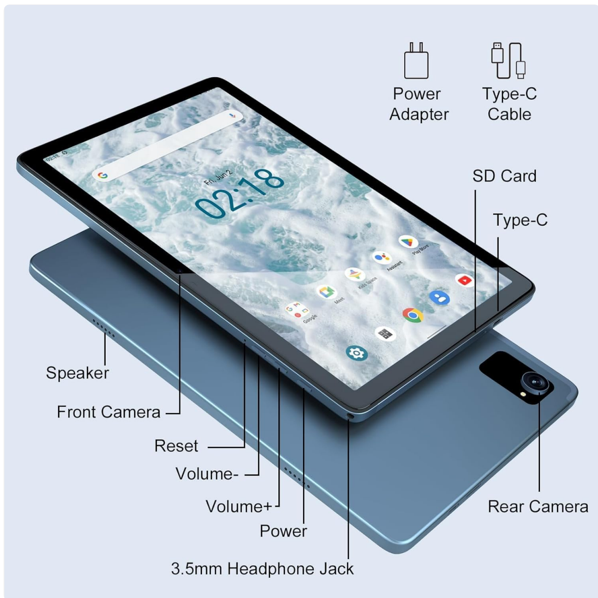
Image 2.2: Detailed view of the tablet's ports and buttons, including front and rear cameras, speakers, and the 3.5mm headphone jack.
