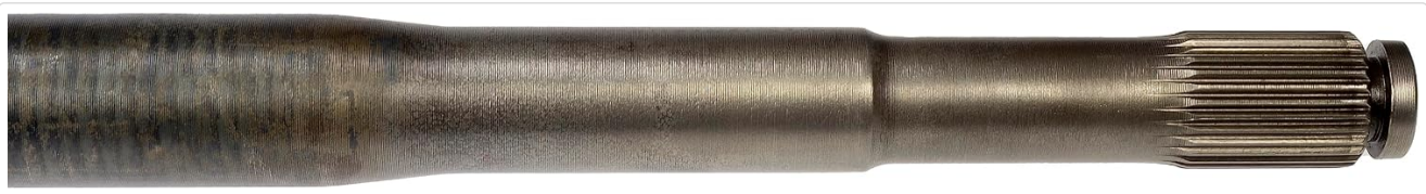
Image 3: Close-up view of the splined end of the Dorman 630-020 Drive Axle Shaft. This end engages with the differential gears.
