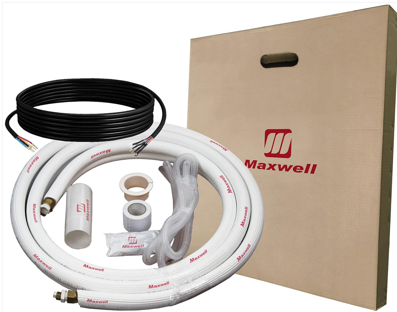
Figure 4: Maxwell 15 ft. installation kit, including insulated copper line sets, communication wires, and drain hoses.
